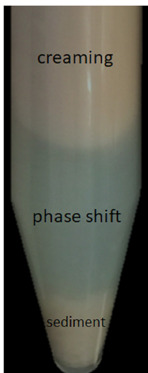
FIGURE 2 Illustration of creaming, phase shift, and sediment to calculate the visual stability index (VS) according to Equation (3)
